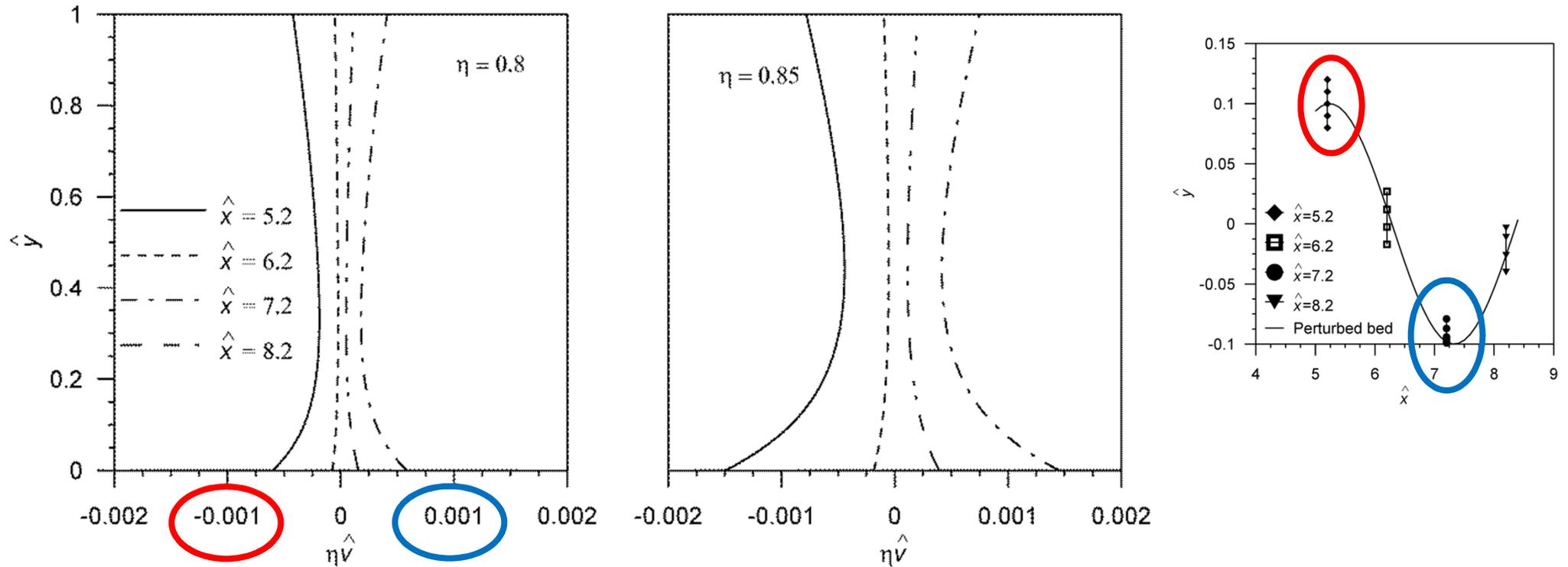
Vertical distribution of vertical velocity at different sections for different  $\eta$
