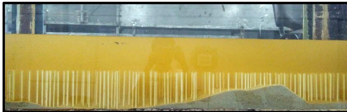
Experiment with submerged rigid vegetation along with sediment transport
