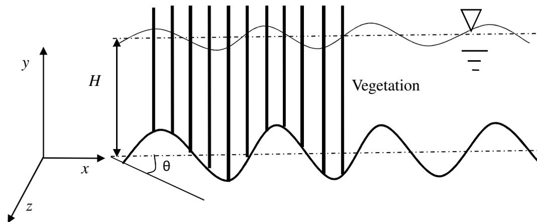
Schematic for flow through emerged vegetation over sinusoidal bed
