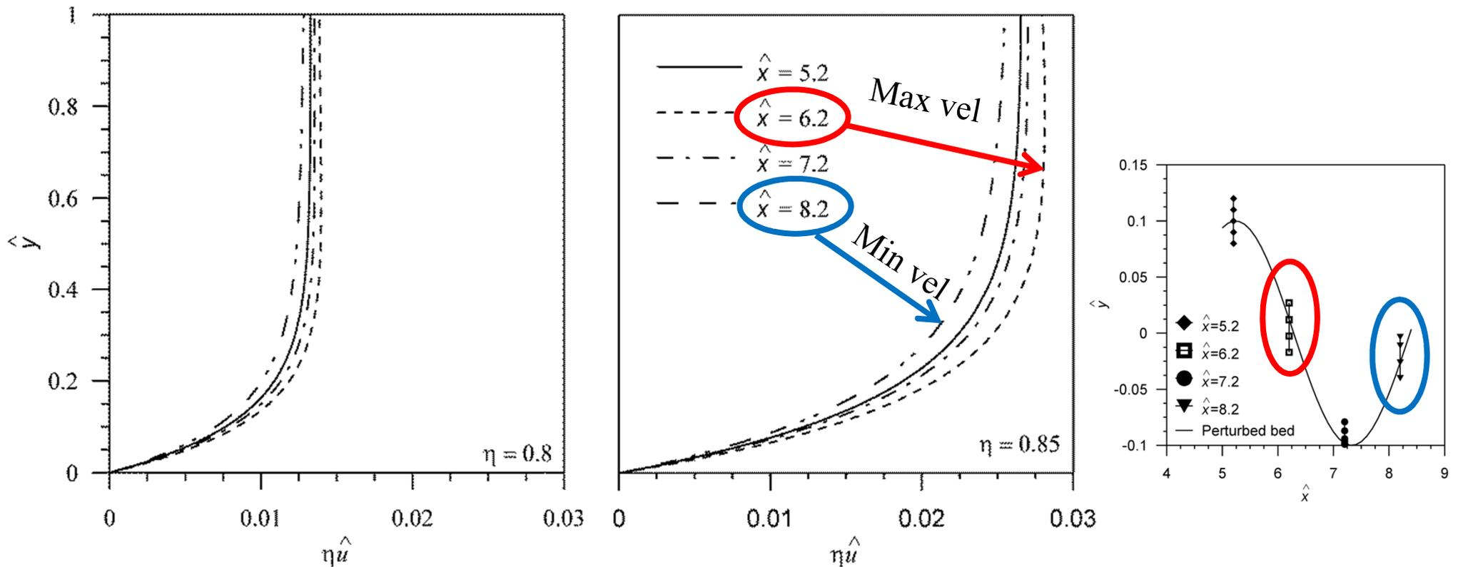
Vertical distributions of longitudinal velocity component at different sections for various  $\eta$
