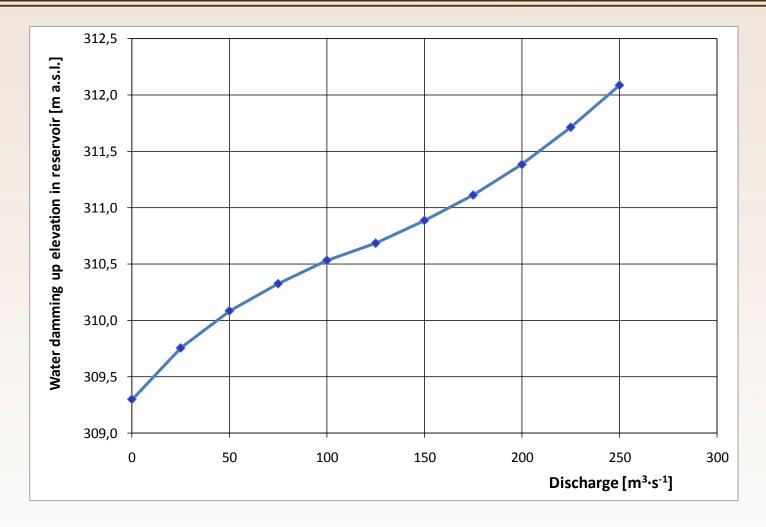
Hydraulic characteristic of side channel spillway of the Złotniki reservoir for the existing state (analytic)
