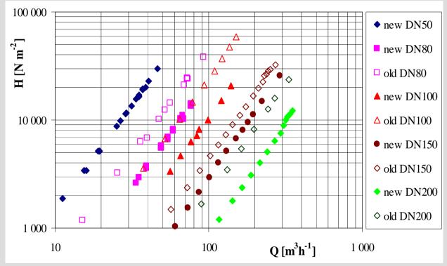
Relation between *H* pressure loss and *Q* flow of old and new filters
