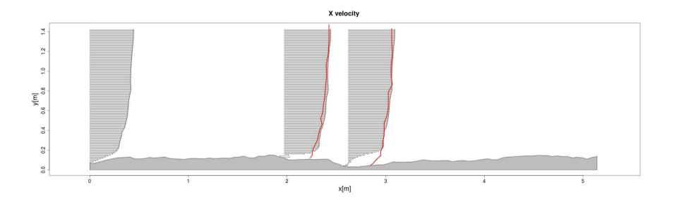
Mean velocity distributions do not fit the field measurements data in the trough and in the lee part of bedform
