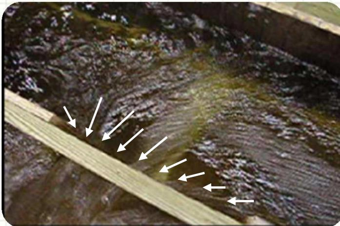
Streamlines direction and rough relative velocity at exit section at flume side breach,  $Q_u = 0.16\text{m}^3/\text{s}$ ,  $Q_r = 0.8$ ,  $Z = Z_{\text{surface}}$
