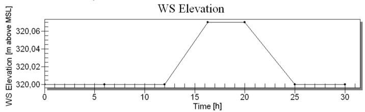
Water surface boundary condition for dynamic simulations. Damping water from the upper tank causes a 7 cm WSE rise in the lower tank.
