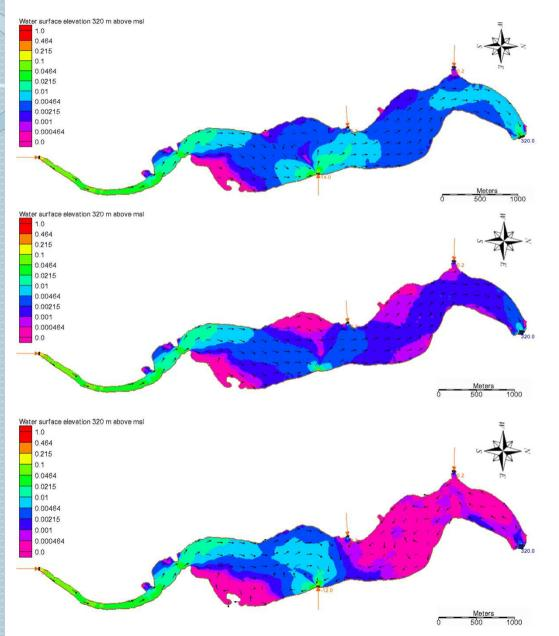
Planar velocity fields resulting from steady state simulations for 8.7 m<sup>3</sup>/s main inflow:
