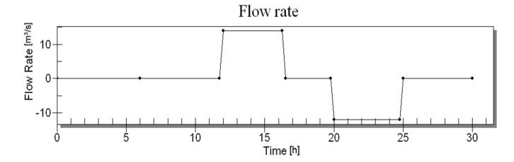
Power plant outlet discharge rate boundary condition for dynamic simulations. Pumping water upwards takes a longer time as the discharge value is lower.
