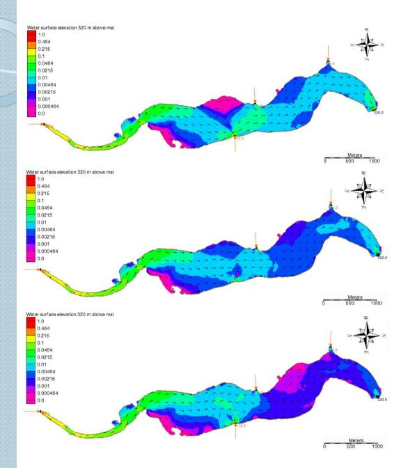
Planar velocity fields resulting from steady state simulations for 20 m<sup>3</sup>/s main inflow:
