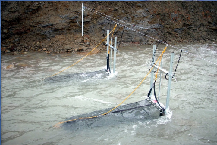
Two River Bed load Traps installed at Scott River (2009)
