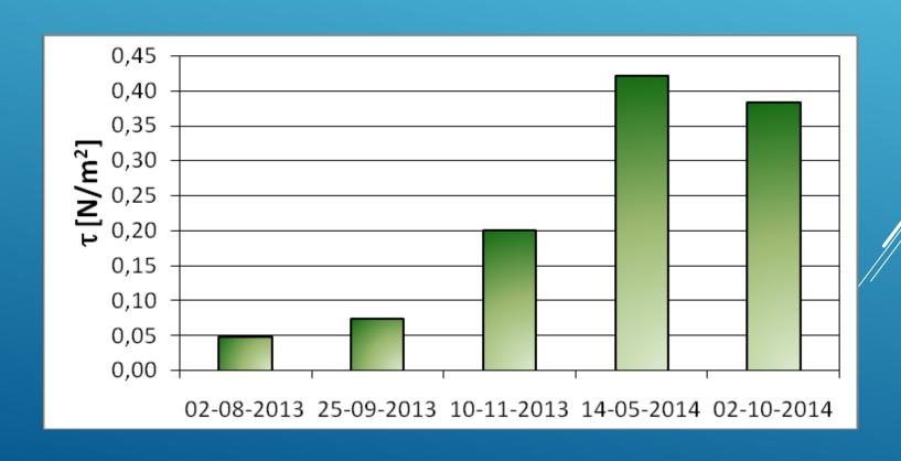
DISTRIBUTION OF STRESS OVER THE REACH WITH INSTALLED PBHS SHORTLY AFTER THE INSTALLATION OF BASKETS AND ONE YEAR INTO THE RESEARCH
