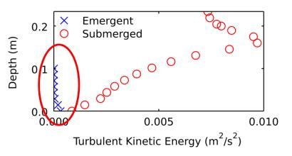
The porous zone approach currently isn't currently suitable as it does not take into account the stem wake effects
