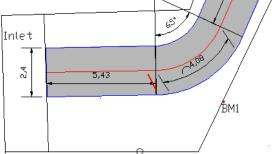
Single groyne installed at the first cross-section
