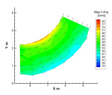
Higher velocity at inner bank due to rectangular cross-section
