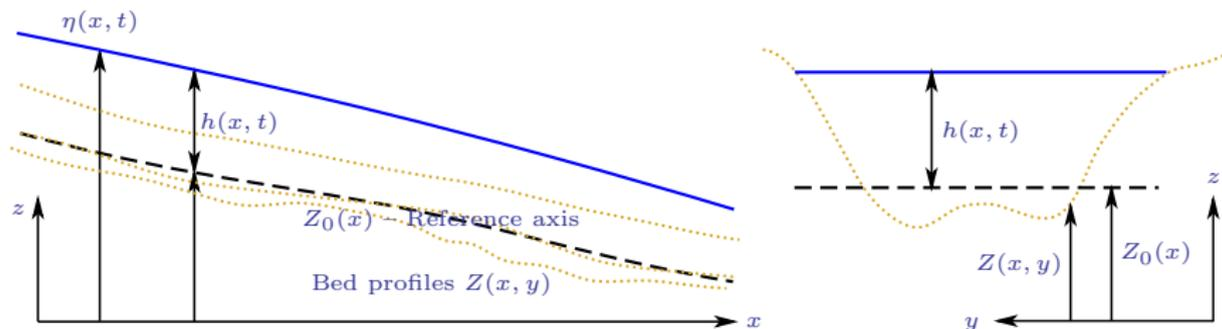
The tradition is not to use  $\eta$ , but instead a depth-like quantity  $h = \eta - Z_0$ , where  $Z_0$  is the elevation of a longitudinal axis, almost always the supposed bed of the channel. The GVFE becomes
