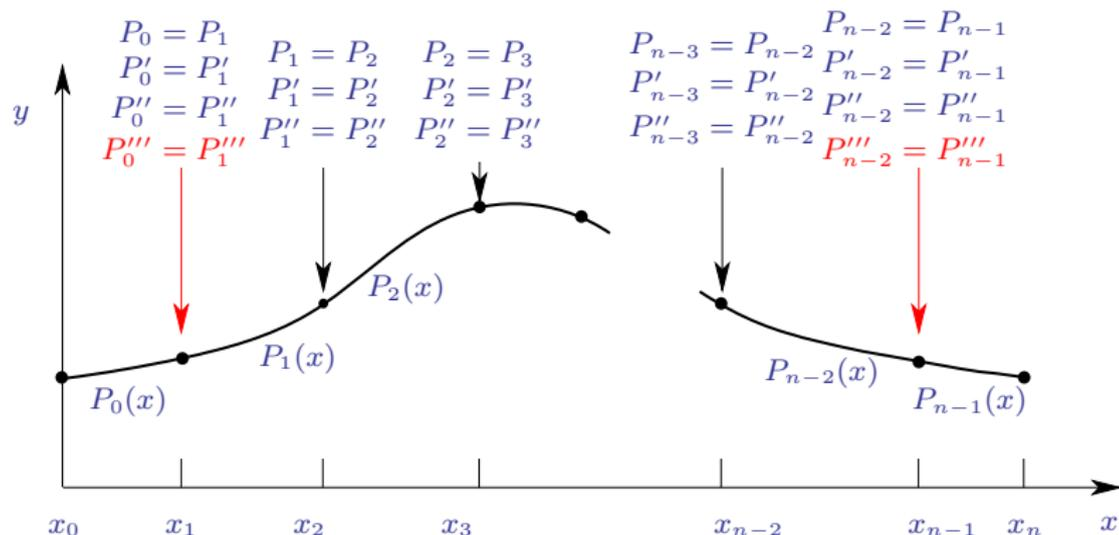
Piecewise-continuous interpolation by cubic splines with not-a-knot conditions shown in red
