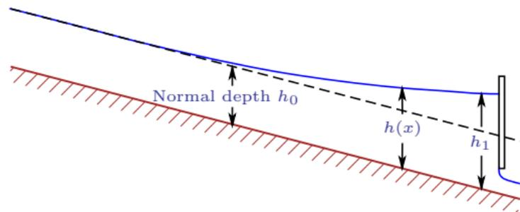
This shows a typical subcritical flow retarded by a structure, showing the free surface disturbance decaying upstream, and if the channel is prismatic, to constant normal depth.
