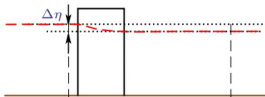
(b) The idealised local problem, uniform channel with friction and slope effects assumed to balance
