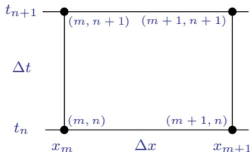
And introducing the more general computational notation with  $Q$  as discharge,  $m$  as space index,  $n$  as time index, and setting  $I_1 = Q_{m,n}$ ,  $I_2 = Q_{m,n+1}$ ,  $O_1 = Q_{m+1,n}$ ,  $O_2 = Q_{m+1,n+1}$  gives the Muskingum finite difference equation:
