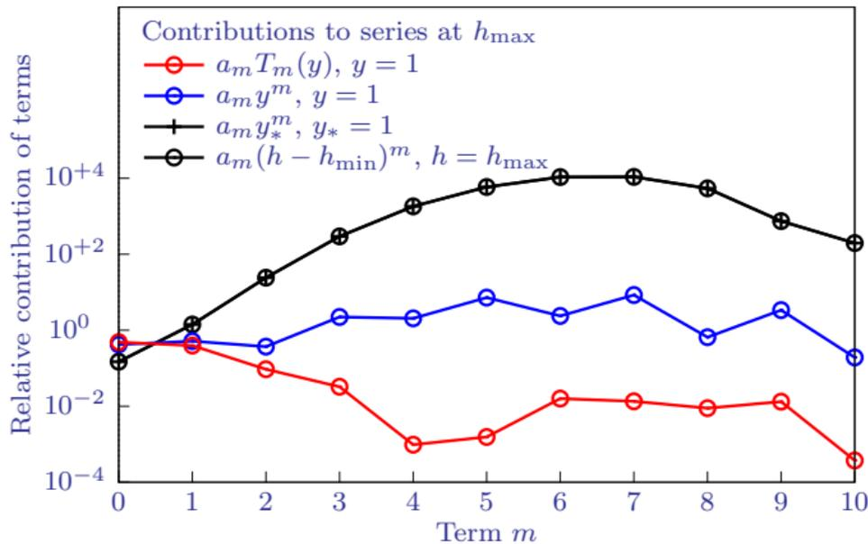
For *global* approximation of data one should use orthogonal functions such as Chebyshev polynomials – or piecewise-continuous splines
