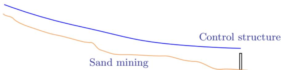
Figure: Typical gradually-varied flow problems – how far does the influence of the control structure extend upstream and/or what is the effect of sand mining?
