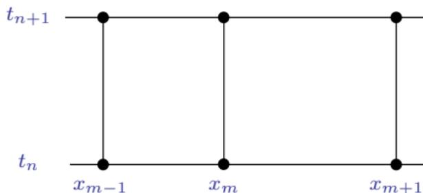
At any of the three computational points  $(x_{m+k}, t_n)$ ,  $k = -1, 0, +1$  we approximate the time derivative by the forward difference approximation
