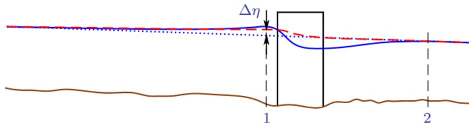
(a) The physical problem showing backwater  $\Delta\eta$  just upstream of obstacle
