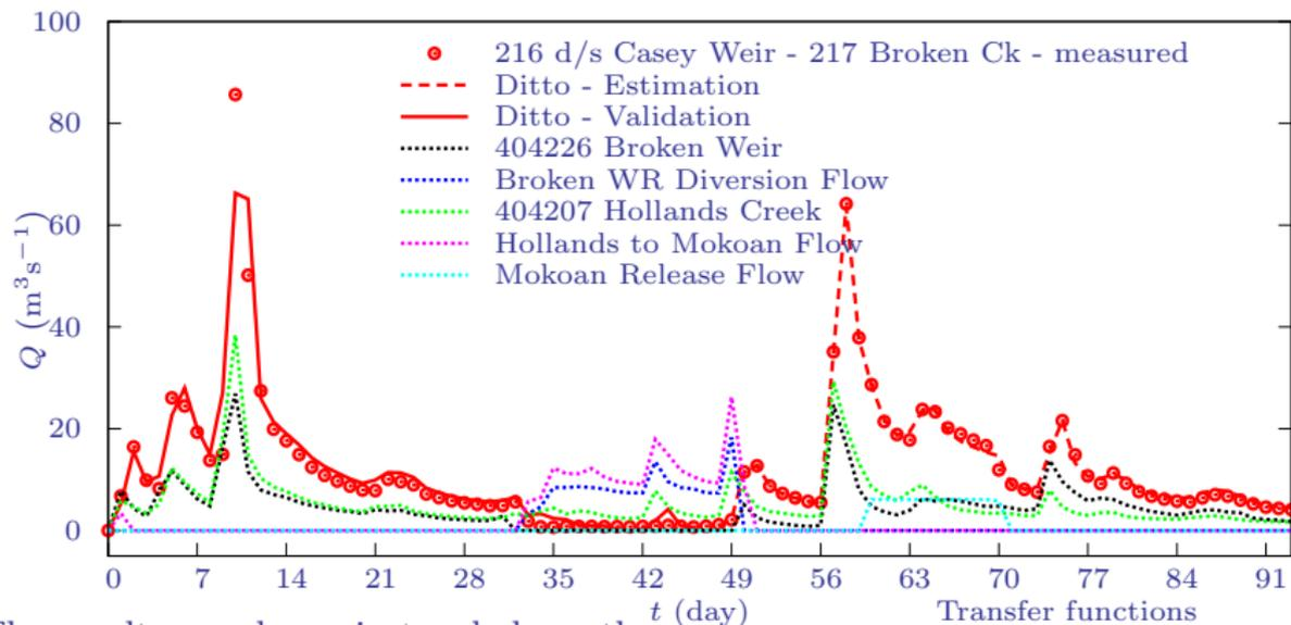
The results are shown in two halves: those for  $t > 45$  d were used to estimate the transfer functions (there was a block release flow from Lake Mokoan between 59 – 71 d whereas there was no release in the other half of the data, for  $t < 45$  d so that it would not have been possible to determine the transfer function for it).
